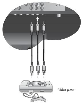
Connect the Composite (AV) output of your AV equipment to the Composite (AV) signal terminal on the TV using a Composite (AV) video cable (RCA connector) as illustrated.
